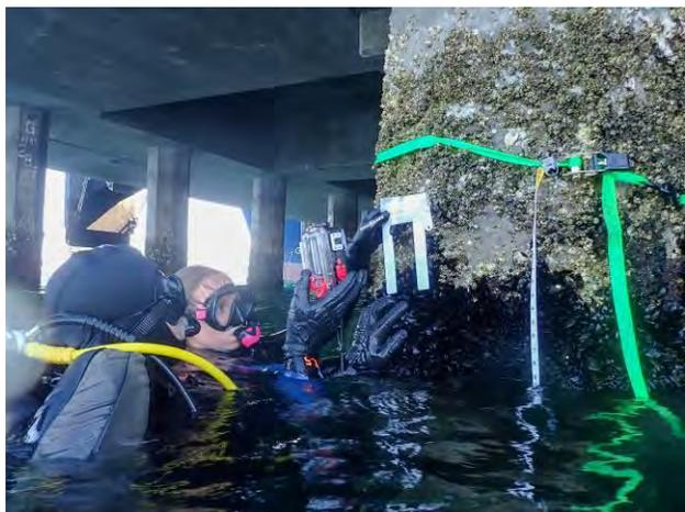
*Divers preparing to collect quadrat scraping in upper intertidal zone on pier piling*
